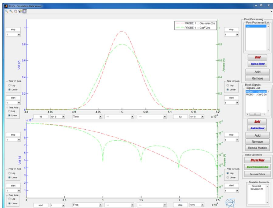
A non-Gaussian bunch shape leads to higher than expected power at higher frequencies.
