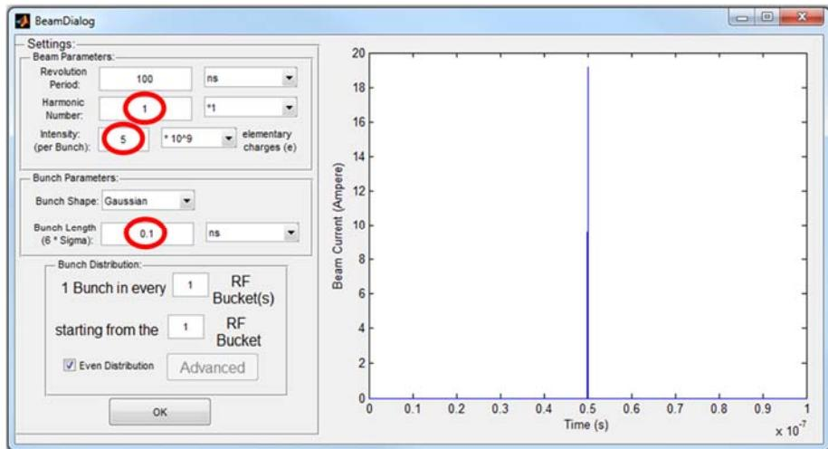
Now put a probe on one of the BPM outputs & simulate the impulse response (you will get an error message to say that the pulse is much shorter than the button and that the simulation may not be accurate – but just click CONTINUE as it's good enough for us!).
