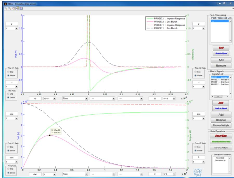
For a  $2\text{ns}$  bunch the high frequency content is defined by the bunch spectrum rather than the button, while the low frequency content is defined by the button. The result is a convolution (multiplication in frequency domain) of the bunch spectrum and the button spectrum. In this case the highest signal is obtained at a frequency of  $330\text{MHz}$ .
