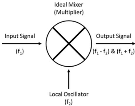
In the most common application, two signals at frequencies  $f_1$  and  $f_2$  are mixed, creating two new signals, one at the sum  $f_1 + f_2$  of the two frequencies, and the other at the difference  $f_1 - f_2$ . These new frequencies are called heterodynes. Typically only one of the new frequencies is desired, and the other signal is filtered out of the output of the mixer.
