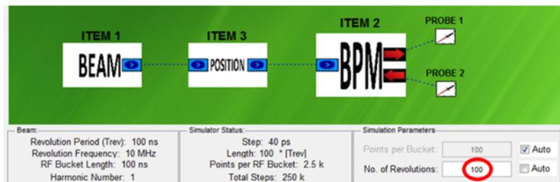
*Use a beam with a 100MHz RF structure comprised of 2ns Gaussian bunches and simulate over 100 turns.*
