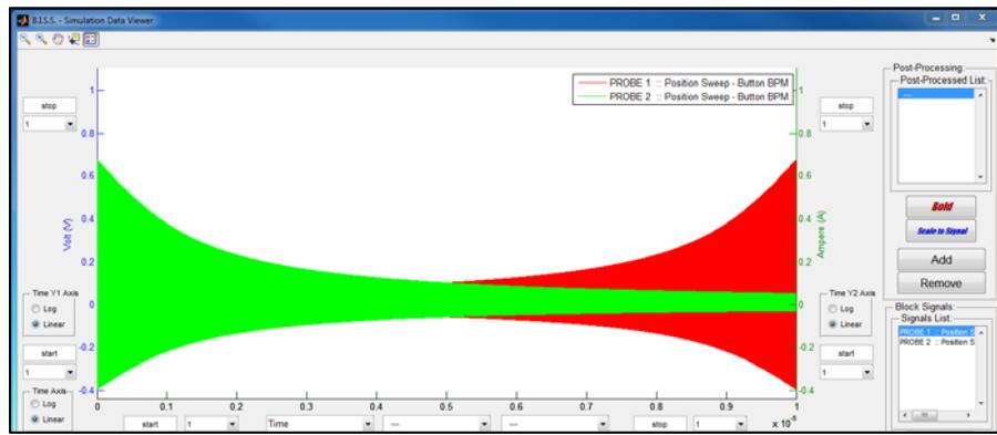
For a button BPM the amplitude of the output increases as the beam approaches the electrode in a non-linear fashion. In this case for a beam in the centre of the vacuum chamber the electrode signal is 100mV, while the signal near the button and on the opposite side is 700mV and 50mV respectively.
