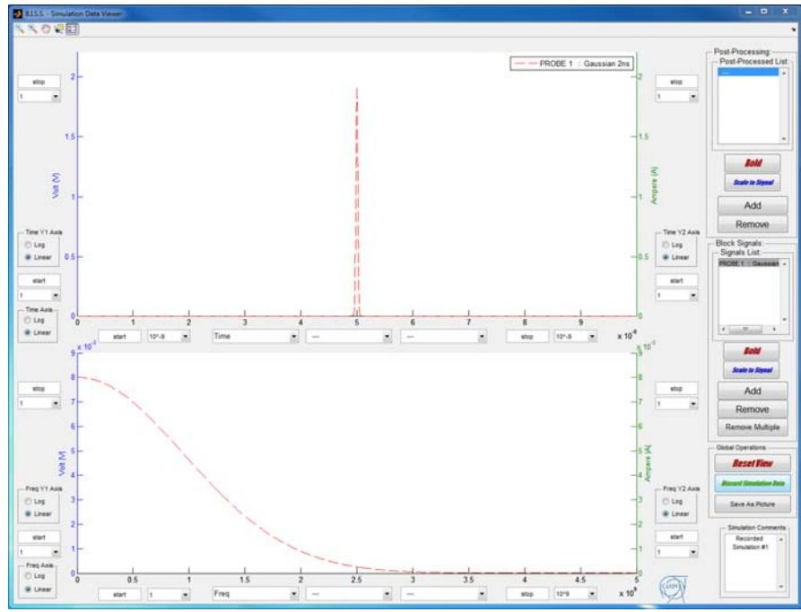
A Gaussian input pulse leads to a Gaussian frequency spectrum.
