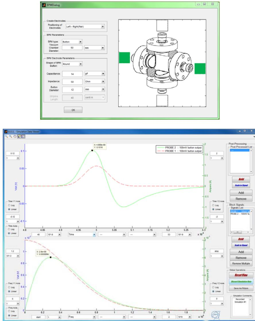
There are many possible combinations. In this example a 14pF button capacitance and a 12mm button diameter is used. The peak output signal is obtained at 290MHz.
