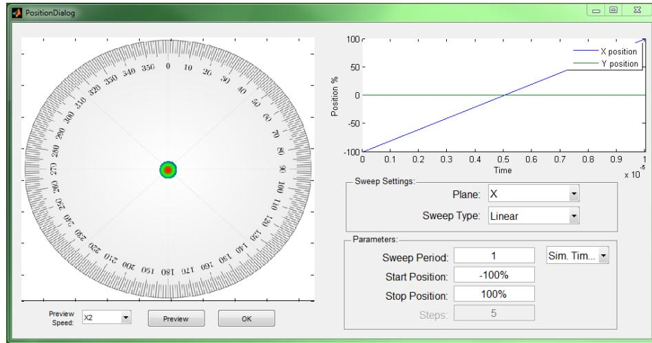
In the example above the properties of the position block are adjusted so as to sweep the position linearly (“Linear” Sweep Type) in the horizontal plane (“X” Plane) from left to right (“Start Position” -100%, “Stop Position” 100%) over the whole aperture. The time it takes to do this is set to be the “Sim. TimeSpan”, i.e. the whole of the simulation time. For a simulation of 100 turns this then gives a position change of 2% of the aperture per turn.
