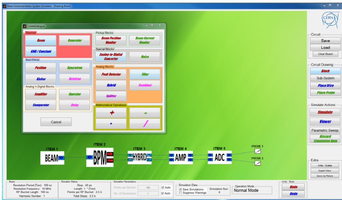
Fig. 1: Workspace with circuit drawing **Block** open
