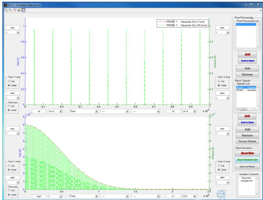
A repetitive signal shows up in the frequency domain as lines at multiples of the repetition frequency. In this case the revolution frequency is 10MHz, so the lines are all spaced by 10MHz. The envelope remains the single bunch spectrum, which still defines up to what frequency there is power in the signal.
