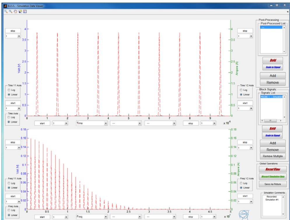
**Fig. 3: The Results Viewer. Top plot shows the time evolution of the signal at a probe, while bottom plot shows the frequency content of the signal for the same probe.**
