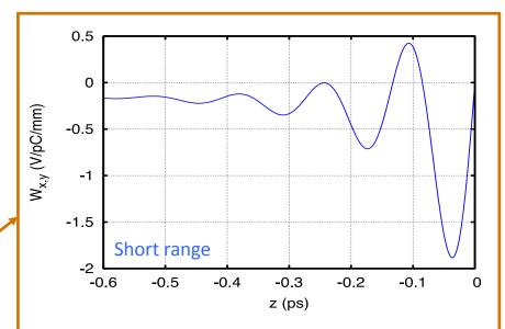
From **behind the source to ~1ps** the wake has an **oscillatory behaviour**, associated to the high frequency resonance
