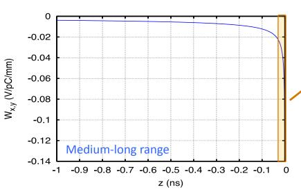
In the range of tenths of ns up to fractions of ms (e.g. bunch length to several turns for the SPS) monotonically decaying wake
