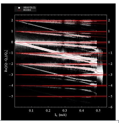
Full calculation for a relatively long SPS bunch (red lines) + macroparticle simulation (white traces)
