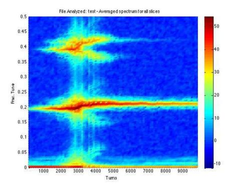
Figure 4: Open-Loop (no feedback) spectrogram of same transient as Figure 3. The beam is TMCI unstable in these conditions,  $\nu_y = 0.185 \nu_s = 0.006$ . Unstable modes 1 and 2 begin at turn 2000 and with charge loss end at turn 4500. Significant intensity-dependent tune shifts are seen as charge is lost in the transient.
