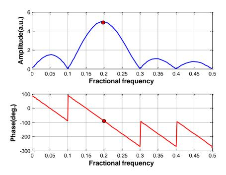
Amplitude and phase response of the filter
