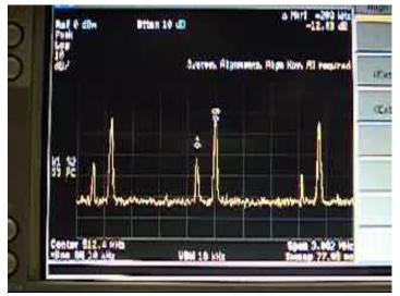
Spectrum analyzer connected to a stripline pickup: observation of vertical instabilities. The sidebands corresponding to vertical coupled-bunch modes disappear as soon as the transverse feedback is activated
