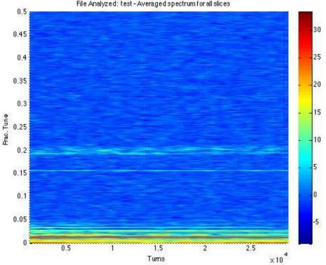
Figure 5: Closed -Loop (feedback on) time-domain recording of bunch motion, bunch samples averaged to show the vertical centroid. The same beam conditions as Figure 3 (TMCI unstable) but motion is controlled by the feedback system. Vertical sensitivity is roughly 14  $\mu$ m/count
