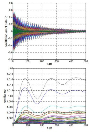
Figure 5: Evolution of single bunch oscillation amplitudes (top) and emittance increases (bottom) as a function of time after injection, using the measured MKI kick.
