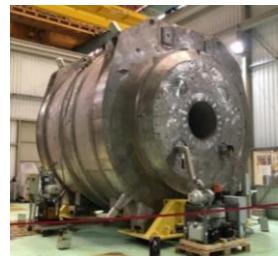
Final leak tests
