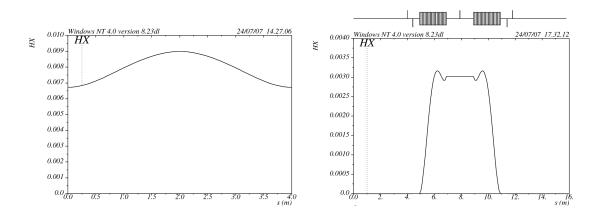
The curly-H function is much smaller in the DBA lattice (right) than in the FODO lattice (left).
