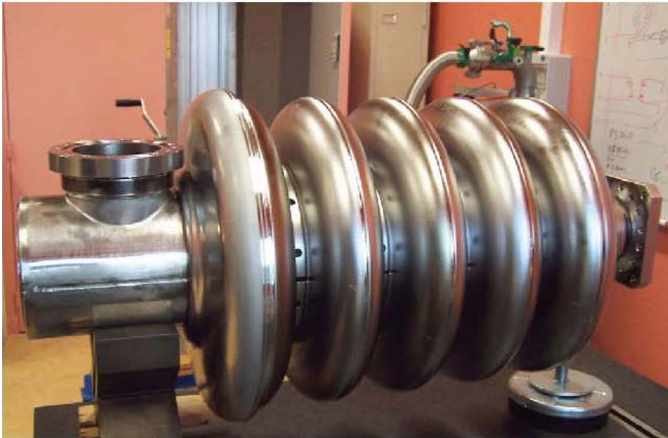
Elliptical 5 cell bulk Niobium cavities (e.g.: \beta=0.47 )
