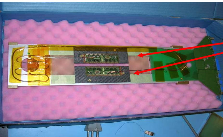
2 Planes with different geometry using ATLAS pixel modules built and operated in NA60 2004 proton run
