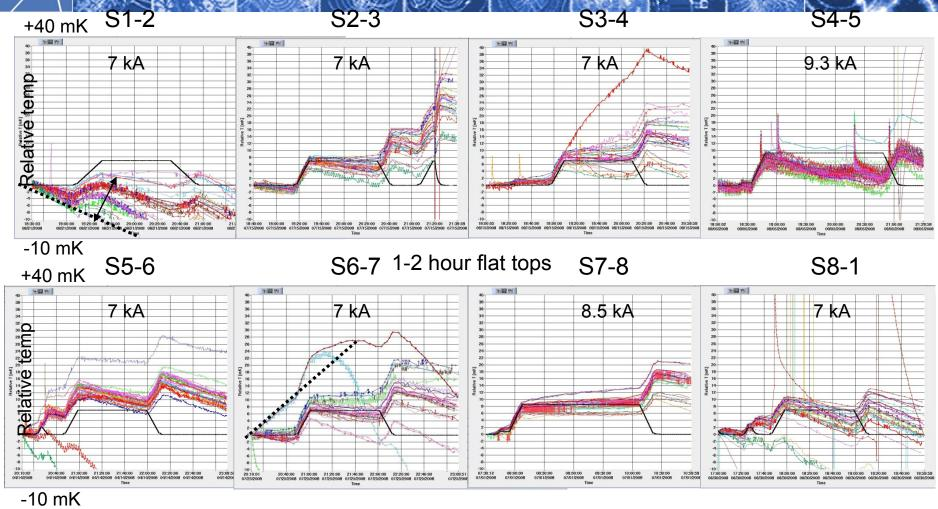
All the current plateaux scrutinized for suspect temperature increase Unstable conditions and dynamic temperature control prevent accurate calculations.
