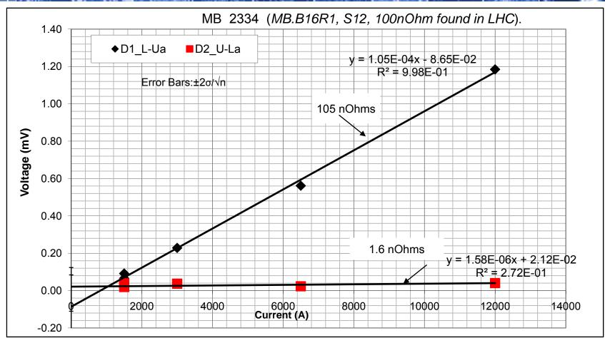
Data from SM18 acquired during the cold tests confirms an inter-pole splice of 105 nOhm in magnet 2334 (B16R1)
