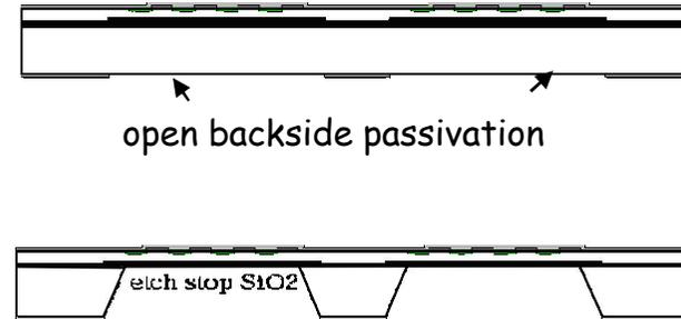
d) Anisotropic deep etching opens "windows" in handle wafer. Structure resist, etch backside up to oxide/implant
