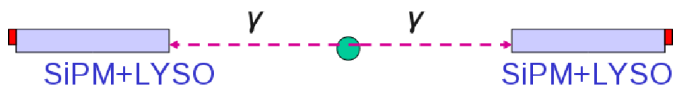
Figure 2: Schematic of the setup used to measure the energy resolution of single SiPMs. A LYSO crystal coupled to a SiPM was used as triggering detector for the coincidence measurement.
