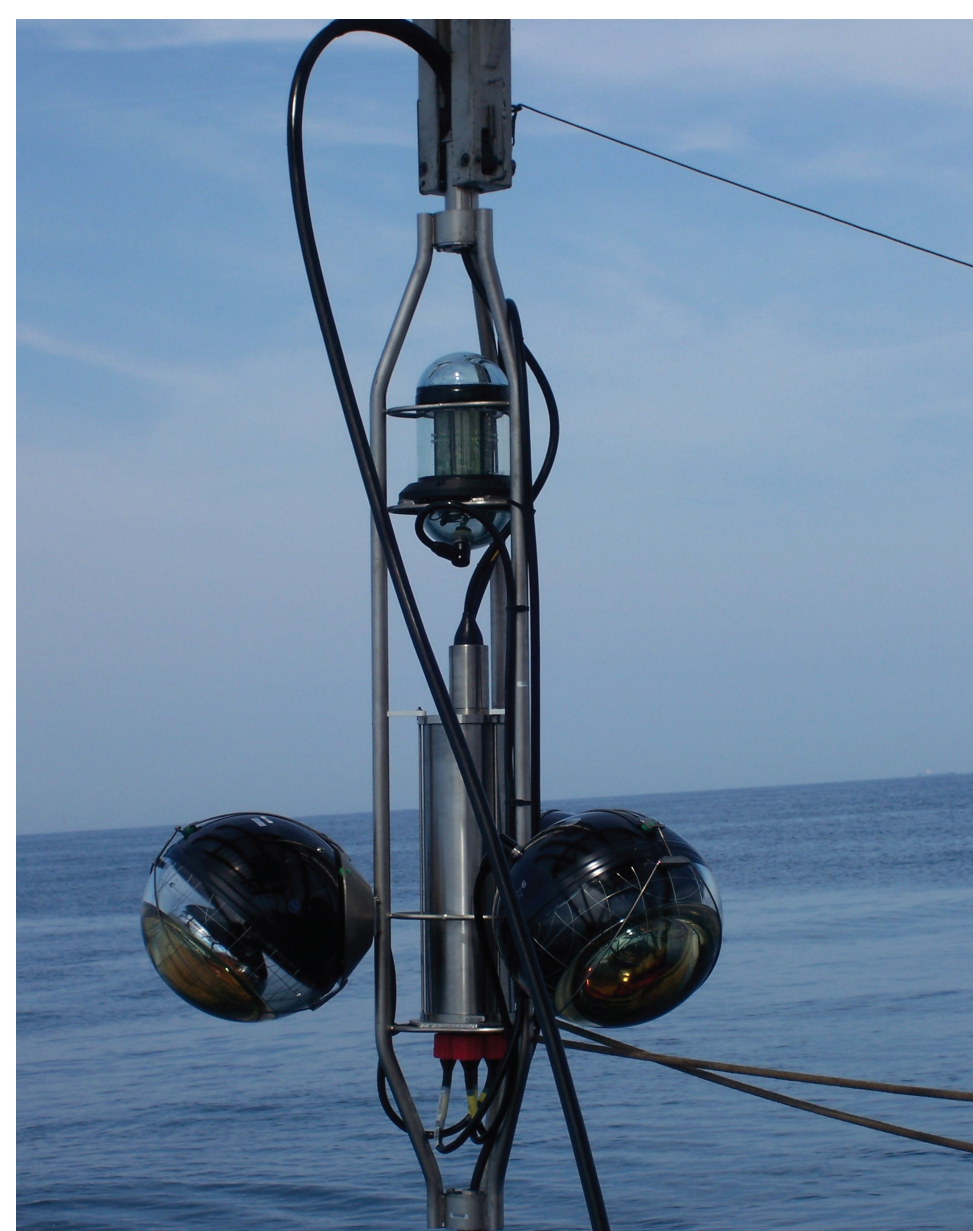
The ANTARES storey carrying three optical modules and the electronics container.
