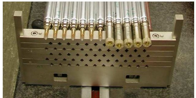
Figure 5: Assembly of a prototype chamber with 15 mm diameter drift tubes. The external endplug reference surfaces at both tube ends are inserted in precise mechanical jigs (before the installation of gas connections and signal caps) in order to position the sense wires with better than 20 \mu\text{m} accuracy.
