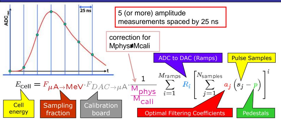
Regular electronic calibration runs (in every fill in when running)
