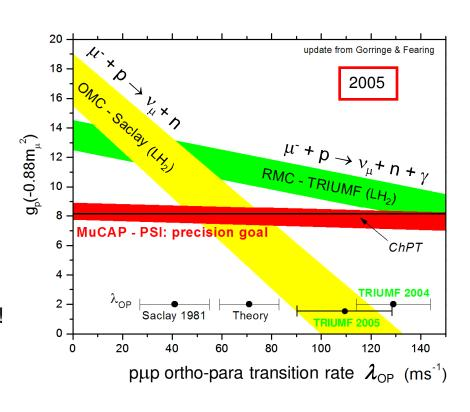
• Realisation: measurement in 10 bar (gaseous)  $H_2$  ( $\rho = 0.012 \cdot \rho_{liquid}$ )  $\rightarrow$  pup formation is slow, all captures proceed from  $\mu p$  singlet state
