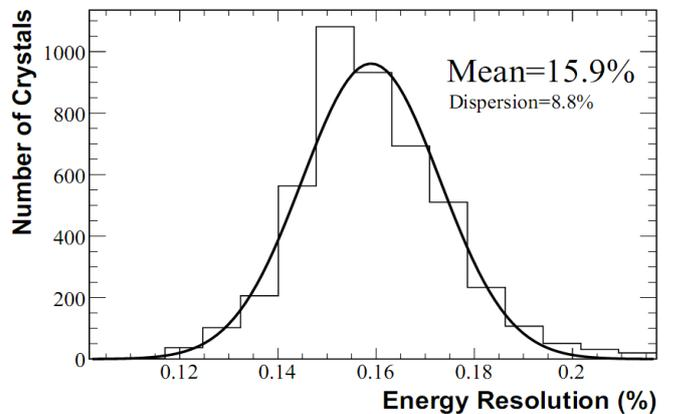
Figure 2: Energy resolution at 511 keV for all channels.
