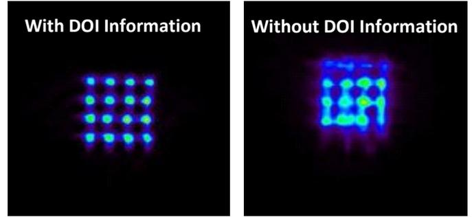
Figure 5: Reconstruction (3D-OSEM) of the  $4 \times 4$   $^{22}\text{Na}$  sources of 1 mm forming a grid with 5 mm pitch, and study of the influence of the DOI information on the reconstructed images (left and right).
