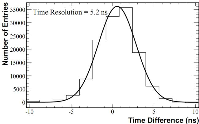
Figure 4: Distribution of the measured time differences between any two hits in opposite detector heads, using a 400 – 600 keV energy window.
