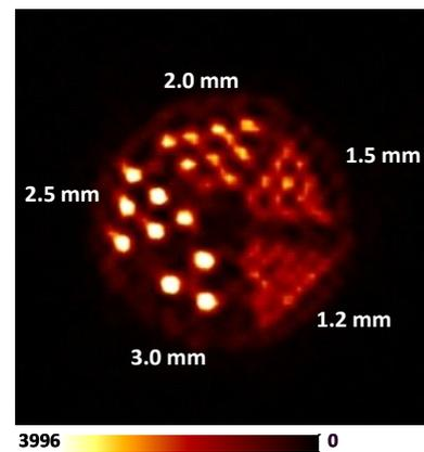
Figure 6: Reconstruction (3D-OSEM) of the Derenzo Phantom.
