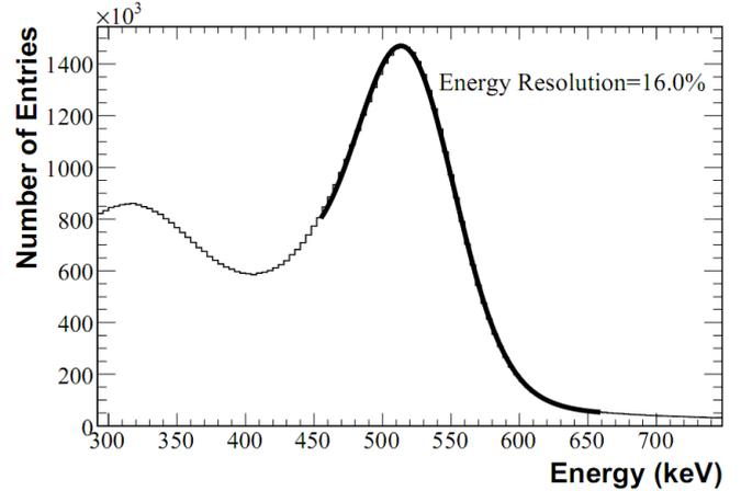
Figure 1: Summed energy spectra of all crystals. The overall scanner energy resolution is 16 %.
