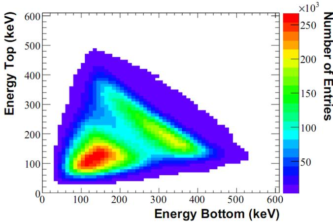
Figure 3: Scatter plot of the crystals top vs bottom event energy deposition.
