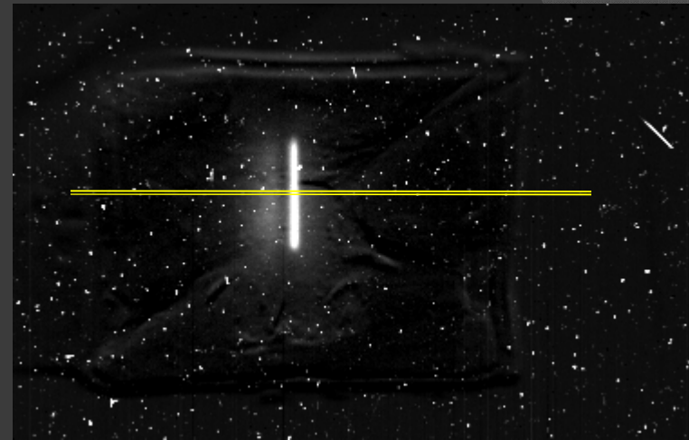
Image of 20x1.6 mm collimator 5 nA beam current, 3 s exposure
