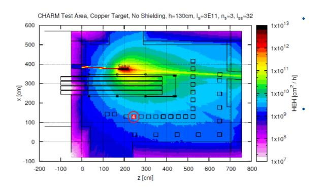
The CHARM radiation levels are simulated using FLUKA and benchmarked against measurements (e.g. RadMON)
