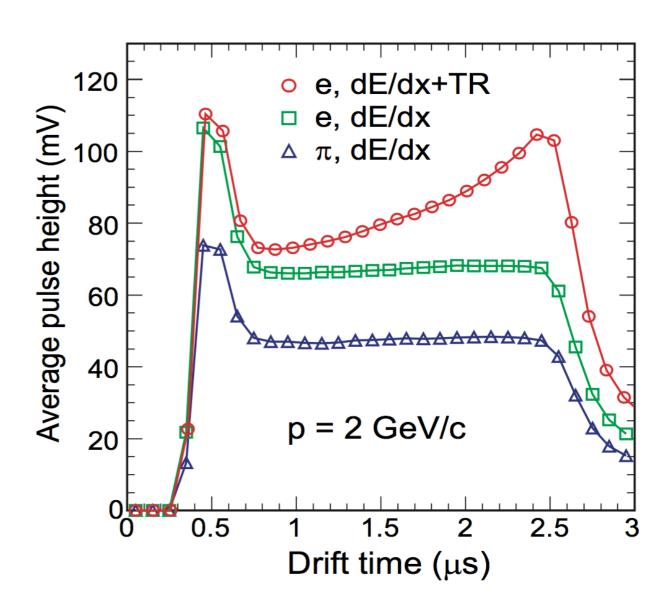
ALICE TRD: stack of 6 identical layers Electrons: larger signal and different time dependence
