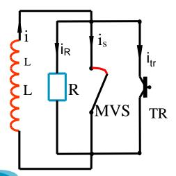
Switch system based on natural commutation, as developed by the Łodz University of Technology
