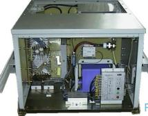
3kV Vacuum circuit breakers family, 250, 400, 800 A for electrical railway traction vehicles (ŁUT, Łodz, Poland)
