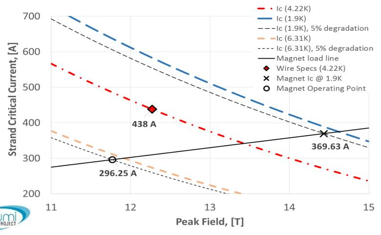
4.4 K Temperature Margin; 20 % Margin on the Load-Line;  $I_c$  margin about 105%
