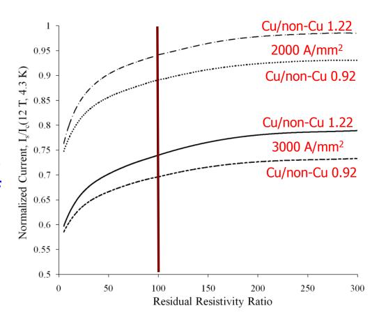
Ratio between the quench current and (12 T, 4.3 K) as a function of RRR in the case of high field instability at 12 T and 4.3 K for different strands.
