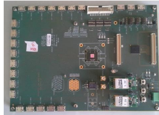
GBTx slave (I2C 16bit reg add, 7 bit chip add)
