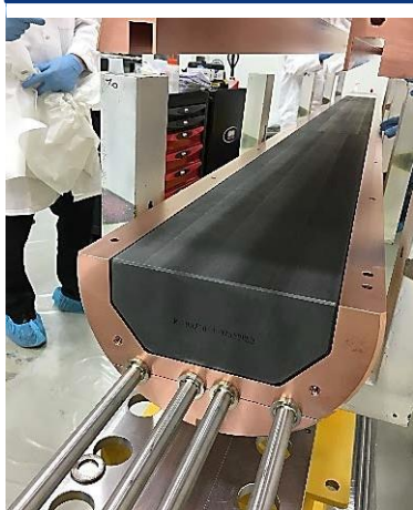
Graphite inside the CuCrZr core
