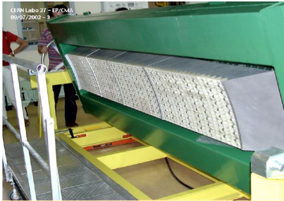
A CMS Supermodule with 1700 tungstate crystals
