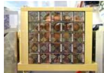
A CMS endcap 'supercrystal' 25 crystals/VPTs
