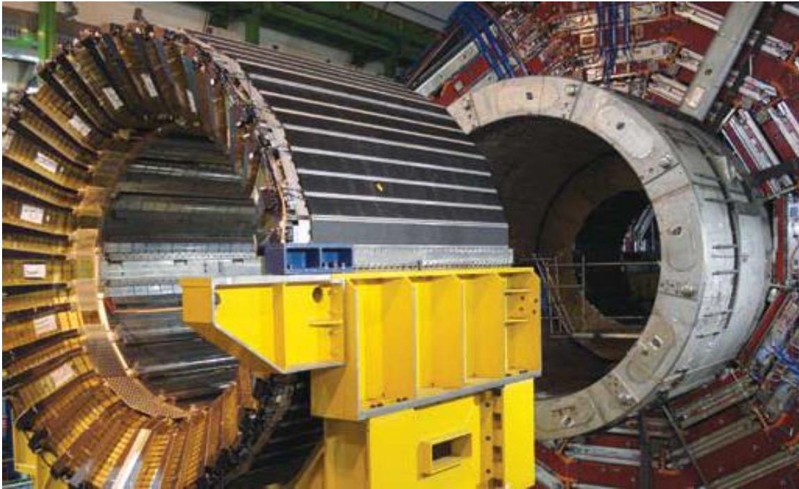
The CMS HCAL being inserted into the solenoid
