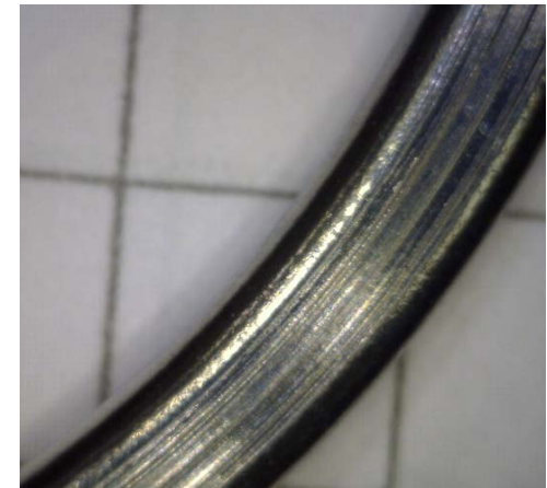
Imprint of machine groove pattern on DN40 Helicoflex® seal (5 mm graph squares)
