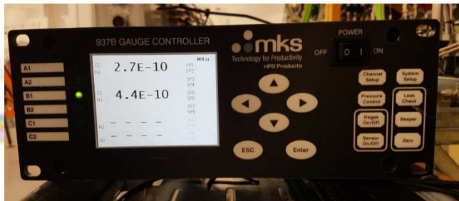
G1 and G2 static pressures (mbar)
