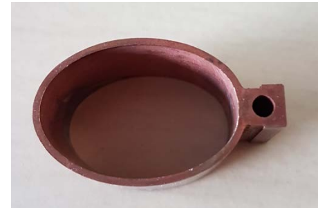
27x18 ellipse section in OFS-copper with e-beam welded cooling channel
