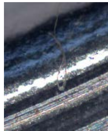
Small fibre (ca 10 \mu m dia) and particle (ca 200 \mu m) on Helicoflex ® seal
