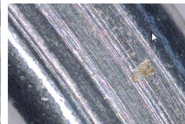
Small fibre (ca 10 \mu m dia) and particle (ca 200 \mu m) on Helicoflex ® seal
