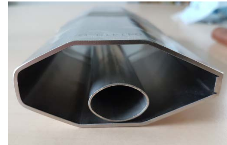
Typical Diamond-I and DDBA vessel cross sections
