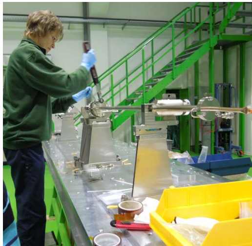
Building up of vacuum strings
