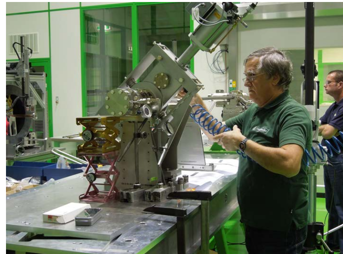
RF gate valve alignment
