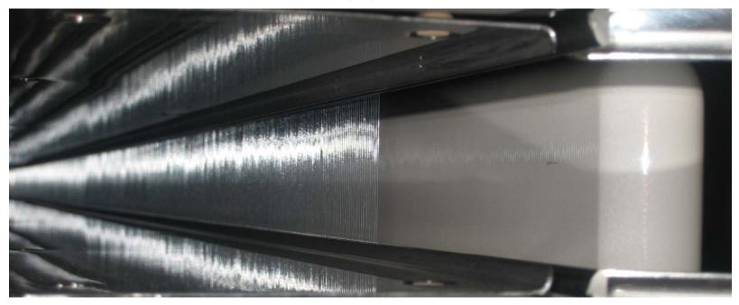
Electrostatic septum (ZS1) wires cut by slow extracted beam (~9x10<sup>12</sup> p).
