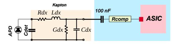
Measured parameters: L = 3,75 nH/cm; R = 0,05 Ω/cm; C = 2,4 pF/cm
