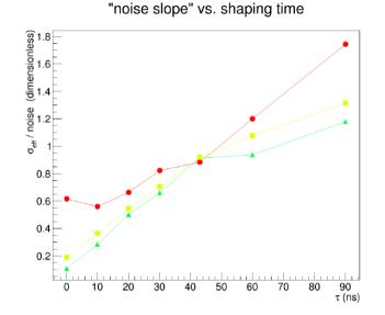
Figure: Here we examine how the dependence of sigma effective on noise (quantified as the slope of the least squares fit line from the above plots) is mediated by pulse shaping time for three sampling periods (red: 25ns; yellow: 12.5ns; green: 6.25ns).
