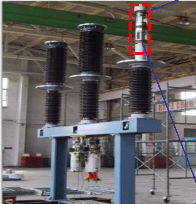
A 126kV single break vacuum circuit breaker Xi'an Jiaotong Univeristy, Xi'an, China
