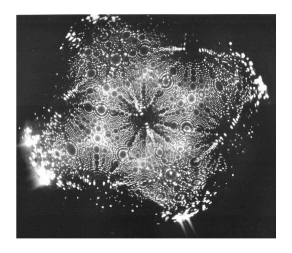
FIM image: Each white spot is a surface atom. The pattern in the image is related to the arrangement of atoms in the tungsten crystal.
