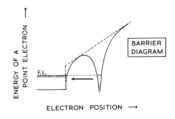
Surface field ionization takes place most rapidly when the topmost electron orbital level in the external gas atom aligns with the Fermi level.
