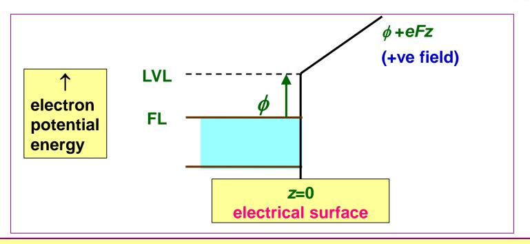
In the limit of large distances z from the emitter, and relative to the Fermi level, the *EEPE* is constructed to have the form
