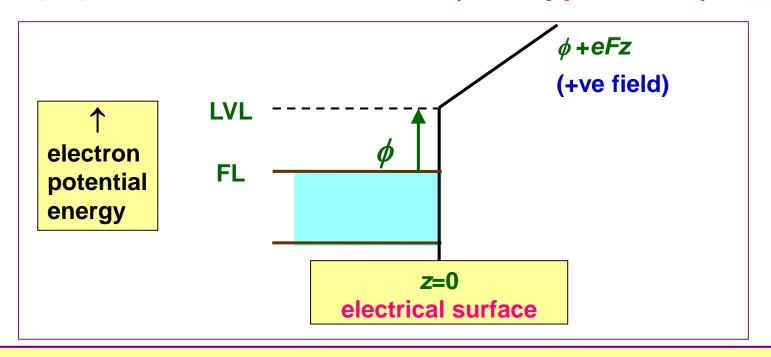
In the limit of large distances z from the emitter, and relative to the Fermi level, the *EEPE* is constructed to have the form
