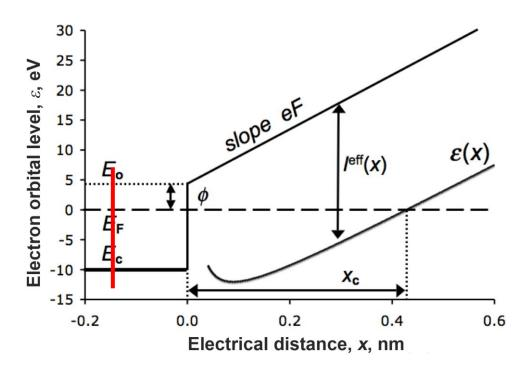
For helium on tungsten, work function = 4.5 eV, ionization energy = 24.6 eV, best image field = 45 v/nm, so critical distance is about 450 pm.
