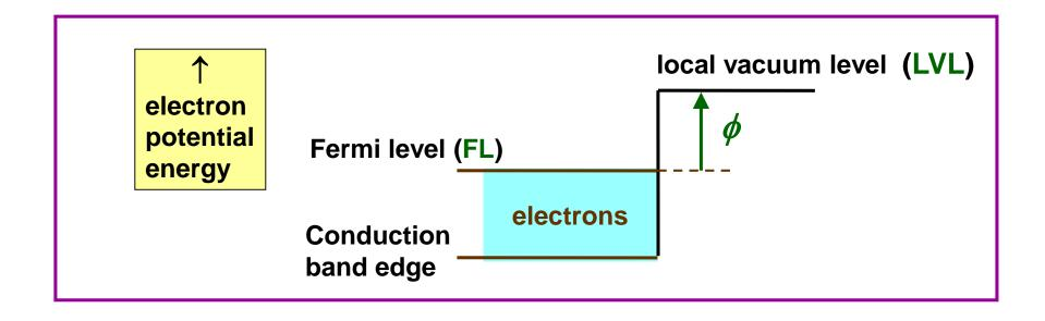
A matter of interest is how the electrostatic component of the total electron potential energy (EEPE) varies with position outside a field electron or field ion emitter surface. The argument is initially presented here for a positive field, but the negative-field case is similar.
