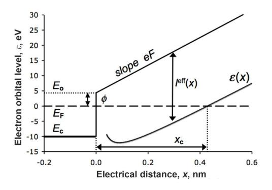
The critical distance is the smallest distance the electrical surface at which field ionization can occur.
