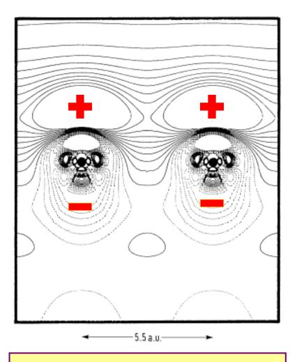
Induced-charge distribution for Ag(001) facet, for an positive external field of 5 V/nm, as calculated by Aers and Inglesfield.
