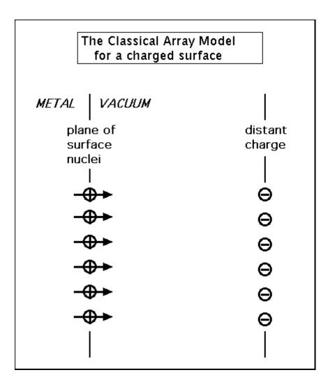
In the planar classical array model, an atomically flat charged surface is modeled by an array of charges & dipoles placed at the positions of the atomic nuclei.
