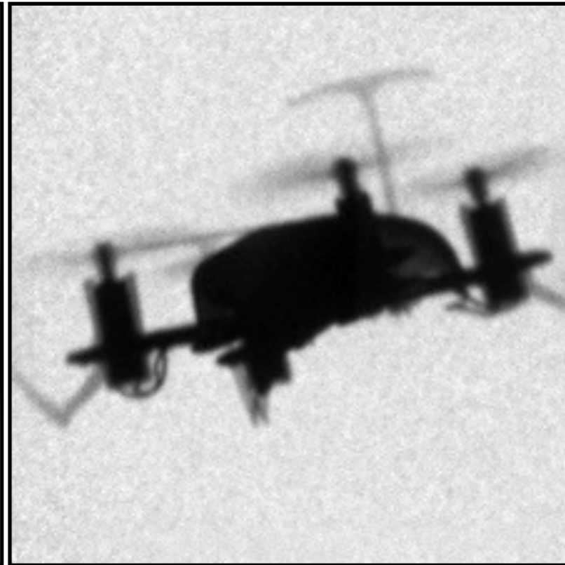
Freeze-frame of an X-ray movie of a flying drone
