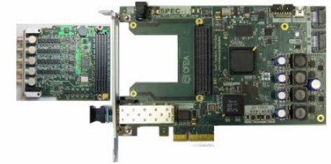
SPEC (Simple PCIe FMC carrier) + FMC (FPGA mezzanine cards) for modular custom electronics.
