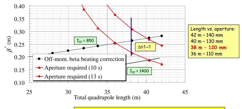
Quadrupole with a 120 mm aperture, 120 T/m chosen for the Phase-I Upgrade
