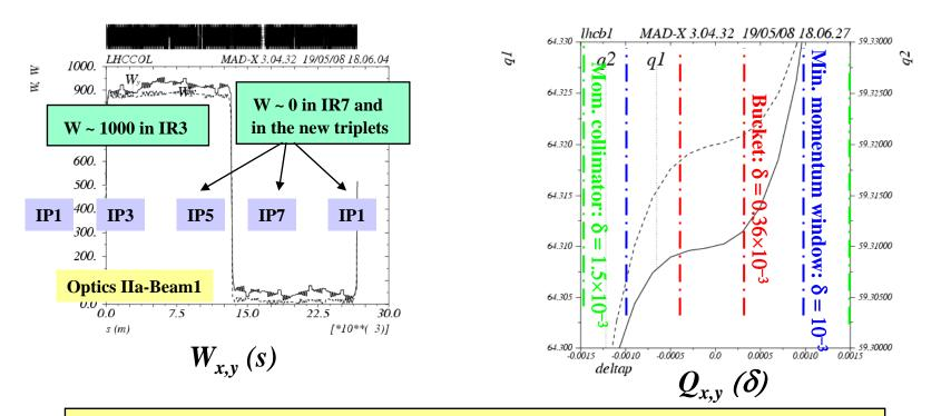
$\Delta\beta(\delta)/\beta(0)$  minimized in IR7 but maximized in IR3 (strong reduction of collimation efficiency).
