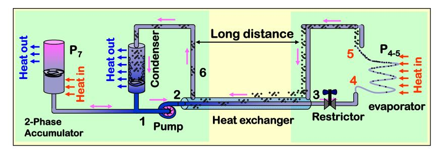
**2PACL (2-Phase Accumulator Controlled Loop) principle of cooling:**
