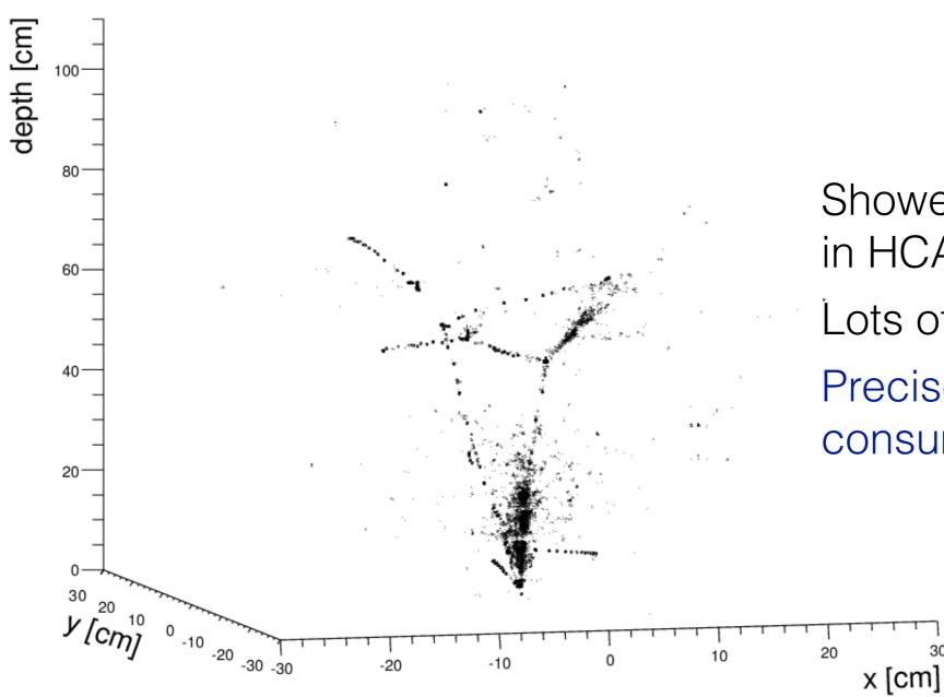
Shower by a 20 GeV pion in HCAL by GEANT4 Lots of fluctuations. Precise simulation is time consuming.
