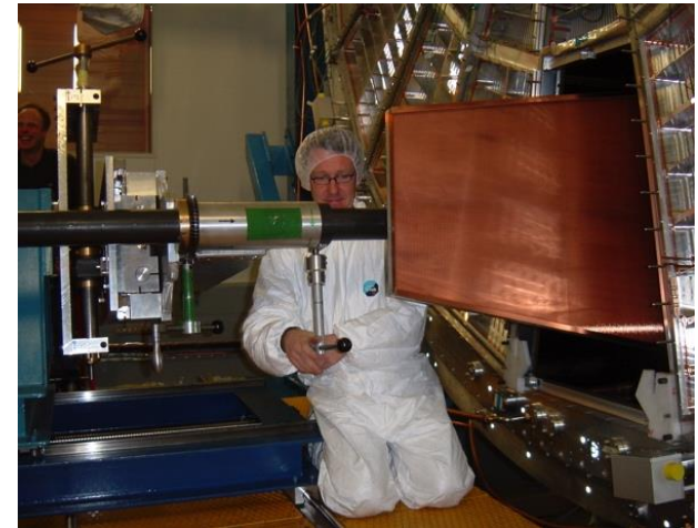
MWPC installation (photo 2006)
