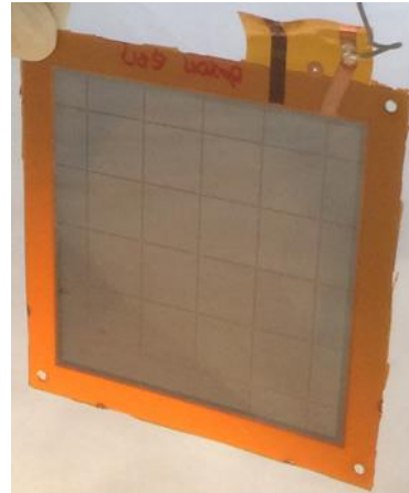
GEM foil 3: top Cr layer is left intact; shadow of evaporated bottom layer can be seen
