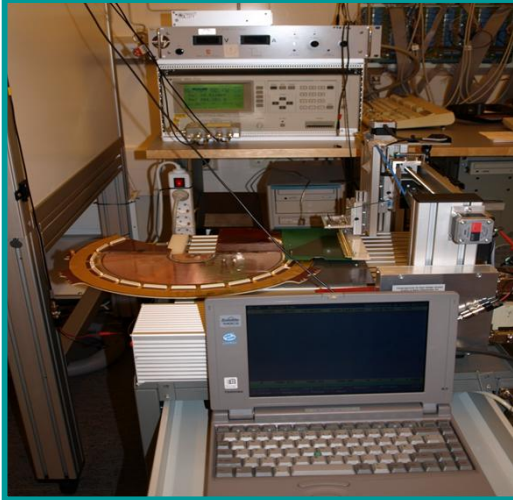
Readout Board Capacitance Distribution Connector 128 strips
