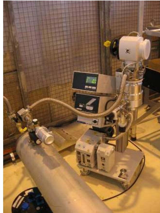
Low Current Module of Cryogenic Electrical Feedbox under pressure and helium leak tightness test
