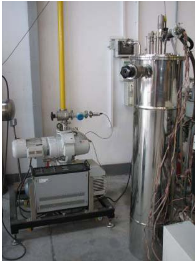
External vacuum jacket during leak test
