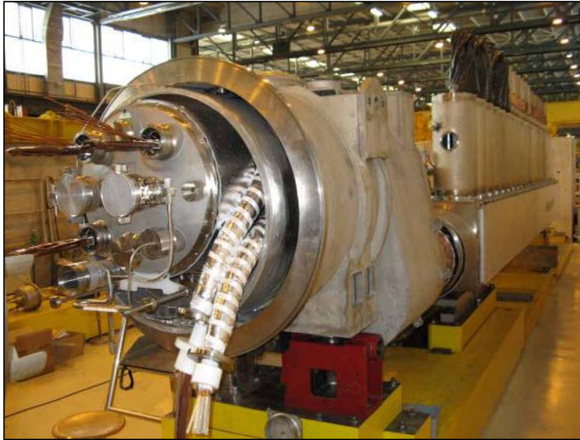
High Current Module of the Cryogenic Electrical Feedbox (DFBAC) during preparation for the pressure and helium leak tightness test
