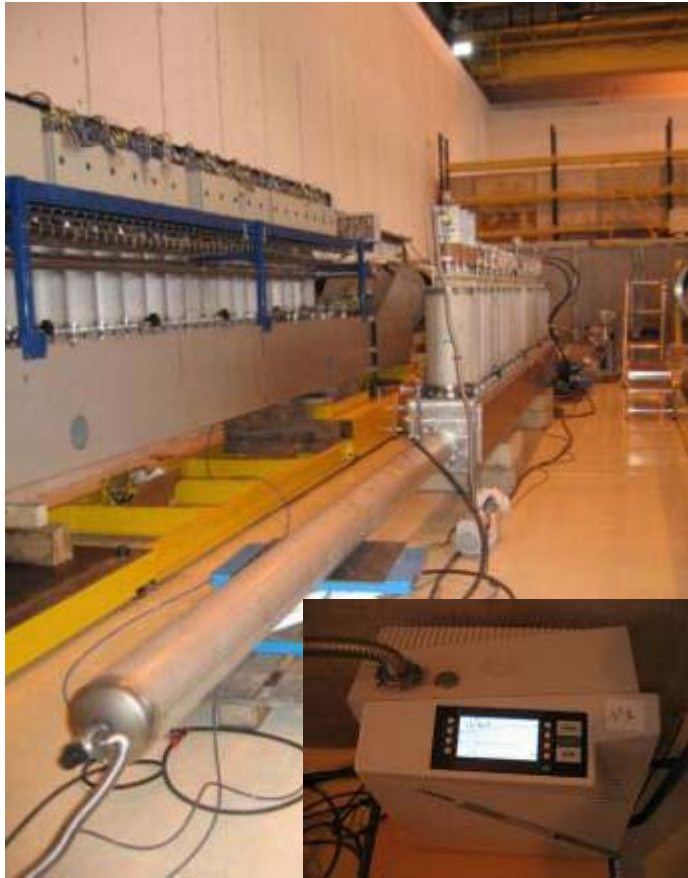
Low Current Module of Cryogenic Electrical Feedbox under pressure and helium leak tightness test
