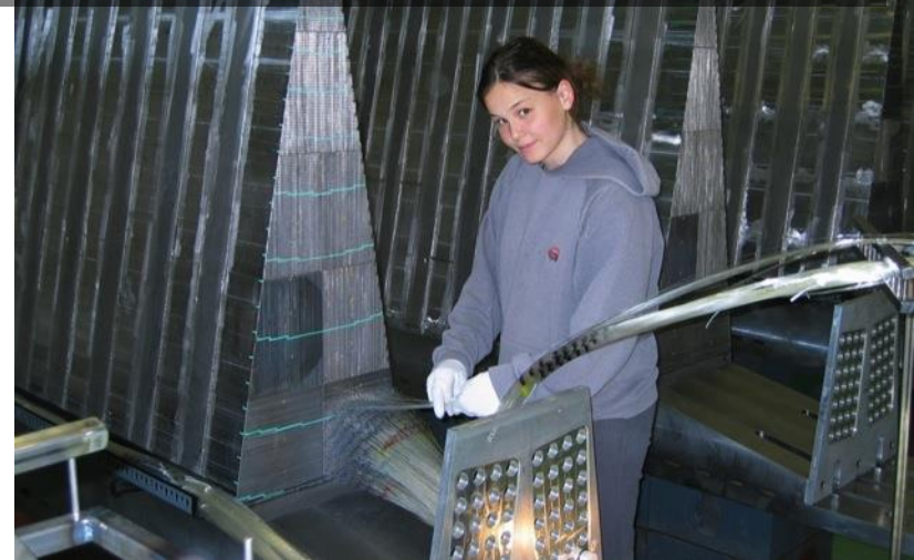
Inserting quartz fibres into a steel wedge
