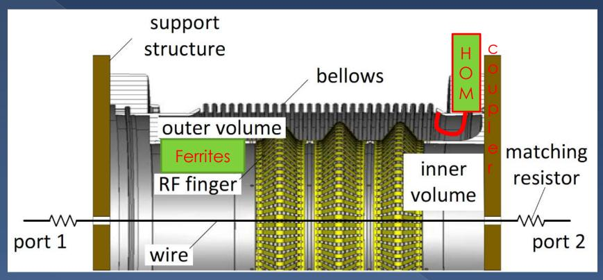
If the high-Q resonances from the outer volume pose a problem, we propose to consider damping in-situ with absorbers or with a small HOM coupler. Thank you for your attention!
