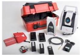
Specifications for precision Leica AT402 15µm + 6µm/m MPE 7.5µm + 3µm/m typical → Precision at 10m distance < 0.05mm typical (1 sigma)
