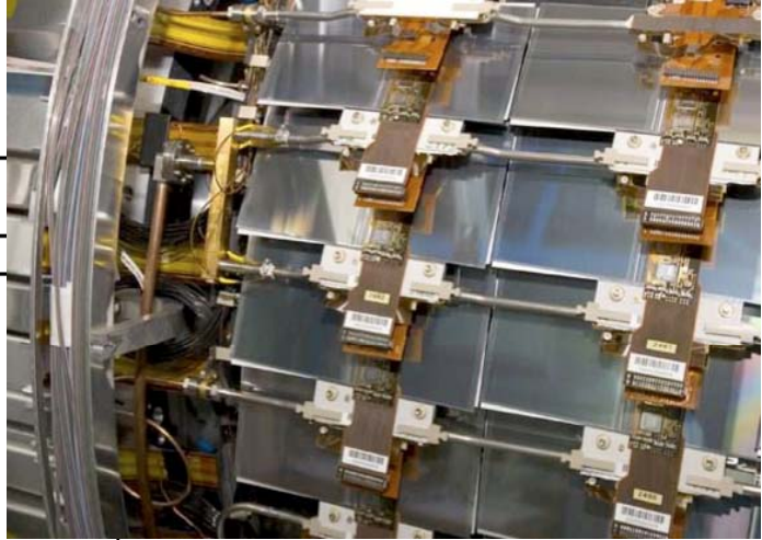
4088 modules, 80 \mu\text{m} micro-strips 61\text{m}^2
