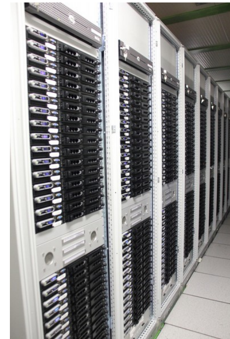
Typical HLT node: 2x12-core Intel Xeon Haswell → 96 cores/box 48 GB RAM, 10Gb Ethernet 4 motherboards in 2U box
