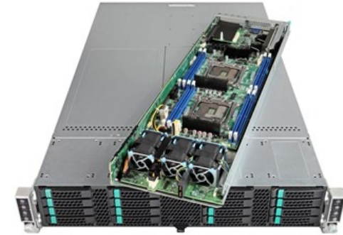
Typical HLT node: 2x12-core Intel Xeon Haswell → 96 cores/box 48 GB RAM, 10Gb Ethernet 4 motherboards in 2U box
