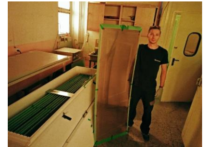
ALICE production: more than 40 GEM foils produced Production rate 36 GEM/month
