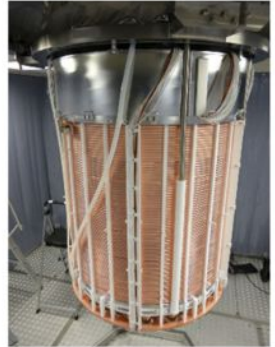
Fig. The XENON1T time projection chamber prior to installation at LNGS, November 2015.
