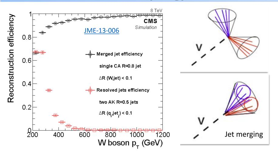
In the searches for resonance with mass heavier that 600 GeV it is critical to use boosted analysis technique.
