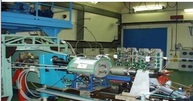
1 MeV neutron displacement damage tests
