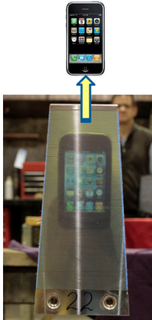
Completed BCAL module. The iPhone is placed against the opposing surface of the 4 meter module.
