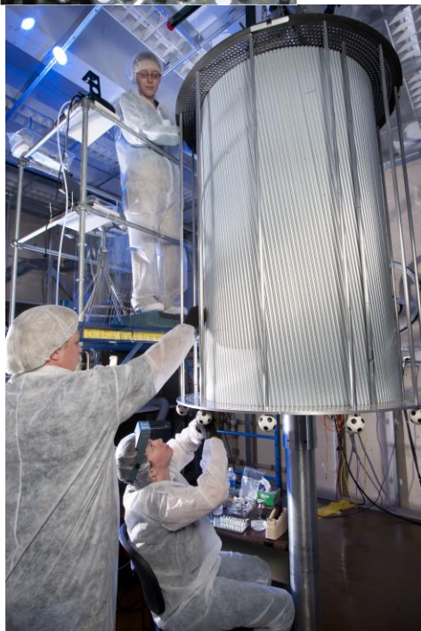
The Central Drift Chamber (CDC) being constructed at Carnegie Mellon University. Construction is done with the device in the vertical position, but it will be turned sideways for installation.
