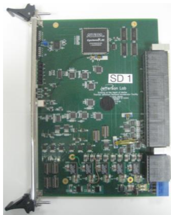
Signal distribution board
