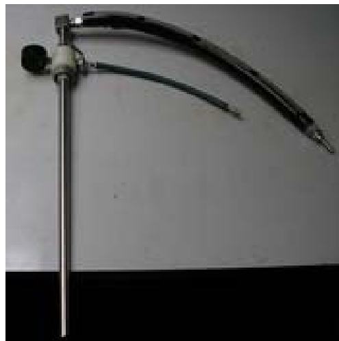
Compressed Air System For pumping of liquid N2 Made in IPNP
