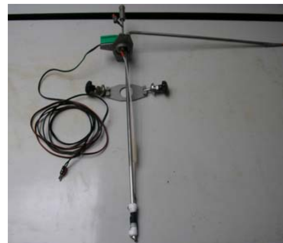
Heating System For Liquid N2 vaporization Made in Cryocom comp. Modified in IPNP
